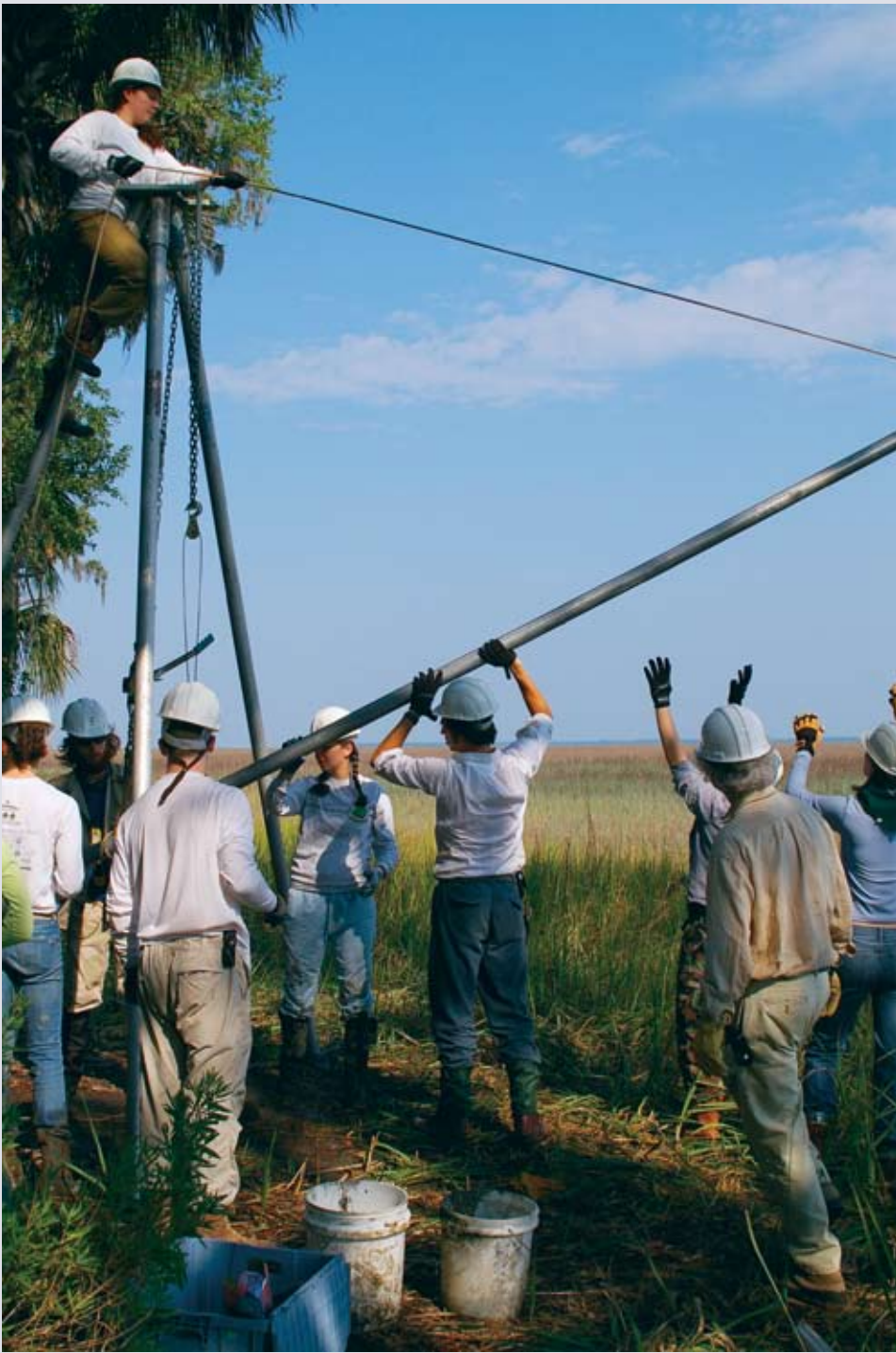
Above: Students used a vibracore to take geological samples up to 20 feet deep. Right: Tim Keith-Lucas, Island Ecology Program director, watches as Sally Neas, C'08, puts some muscle into the work. Opposite page: Laurence Hayes, C'07; Allison Laney, C'07; and Eric Keen, C'08, study a transect of saltwater marsh. Students have gathered data on this transect for the last 10 years.
