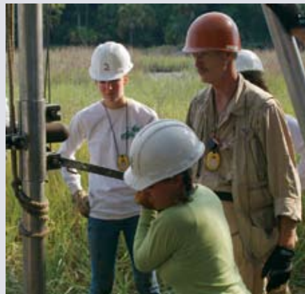
Above: Students used a vibracore to take geological samples up to 20 feet deep. Right: Tim Keith-Lucas, Island Ecology Program director, watches as Sally Neas, C'08, puts some muscle into the work. Opposite page: Laurence Hayes, C'07; Allison Laney, C'07; and Eric Keen, C'08, study a transect of saltwater marsh. Students have gathered data on this transect for the last 10 years.
